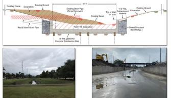
Figure 2: Diagram and photos of changes, General DeGaulle Canal Improvements
