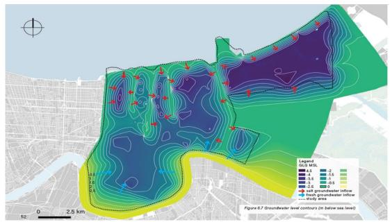
Figure 5-2 Shallow groundwater model generated for New Orleans showing the groundwater flow directions (from areas of light to dark), areas of potential salinization due to saltwater inflow, and areas of freshwater inflow from the Mississippi.
