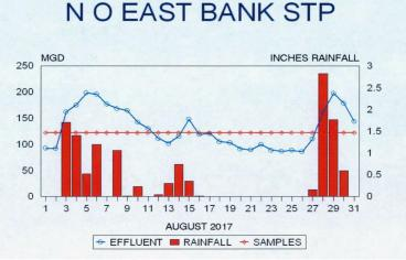
Figure 4-3 Displays the cumulative rainfall per day and the effluent discharge in one section of New Orleans East for the month of August 2017. Effluent increases correlate with rainfall events as groundwater height is increased and subsequent pressure change allows for more water to enter the wastewater discharge network.
