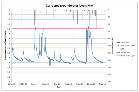
Figure 6-1 Groundwater fluctuation in relation to precipitation events in an observation well in the center of Mirabeau. A number of groundwater monitoring wells are already active within the city. The time series indicates that the groundwater level decreases immediately after a rain event towards the depth of storm drainage pipe and sewer pipe below the streets.
