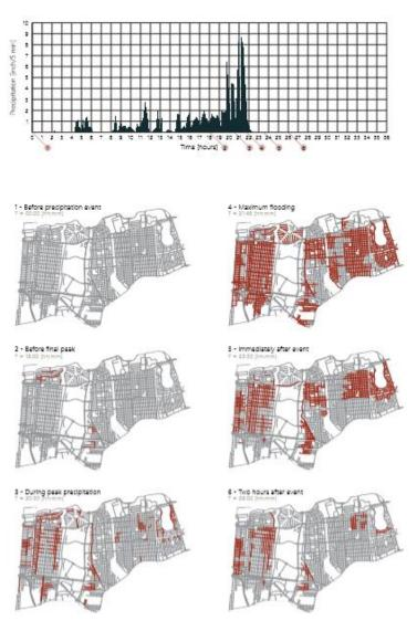
Figure 4-2 The above images were generated with SWMM (Stormwater Management Model) software and shows the effects of a precipitation event on stormwater infrastructure during a given storm (Daan Rooze, 2020).
