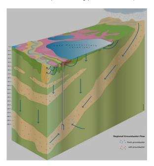
Figure 4-5 A block diagram showing a hydrogeological conceptualization of the subsurface beneath New Orleans. A properly organized and managed groundwater aquifer storage and recovery system could make use of this system, providing a buffer or alternative drinking water source and/or water storage solution.
