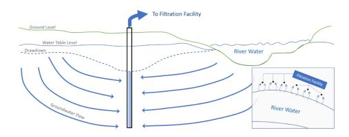
Figure 4-4 Conceptual river bank cross section and infiltration flow lines. Positive effects could include: Groundwater enrichment, natural redox reactions, natural sediment filtration, and biodegradation of contaminants.
