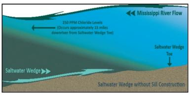
Figure 4-6 Saltwater wedge conceptual diagram shown intruding upstream into the Mississippi River. More dense saline water wedge sits underneath the freshwater river flow.
