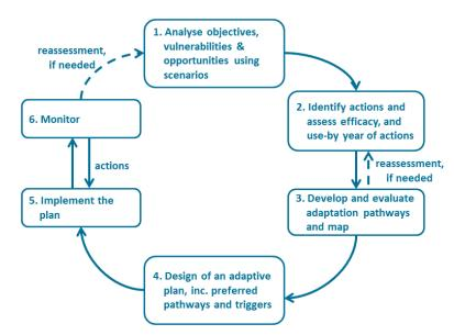
Figure 3-2 The dynamic adaptive policy pathways (DAPP) approach (simplified from Haasnoot et al. 2013)
