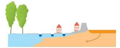
Figure 6-4 (c) Stage 3 – Civil structures and water management practices begin to transform the local ecosystem, reclaiming land by draining a section of the cypress swamp and inducing a flow reversal in the process. Now, the salty groundwater system stemming from Lake Pontchartrain now drains towards the freshwater of the cypress swamp.
