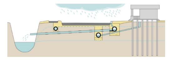
Figure 5-1 Current cross section schematic of the drinking water, sewer and stormwater pipes in New Orleans and associated (low and high) mean groundwater levels.
