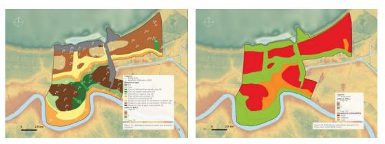
Figure 5-3 (left) shallow soil map displaying types of soil within New Orleans, this information is combined with other to generate the subsidence risk map (right). From the shallow subsidence vulnerability in New Orleans report.
