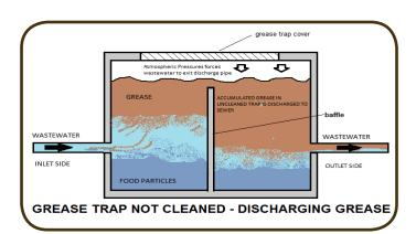
In order to prevent FOG from entering sewer lines and causing backups, grease traps must be inspected and cleaned on a regular basis.
