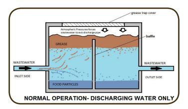
Fats, oils and grease (FOG) are lighter than water and as a result, float. The grease trap has a low inlet pipe and a baffle (barrier) to slow the velocity of the water coming in. This gives time for the solids to settle and the FOG to float.
