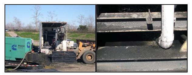
Figure 25. Mobile Dewatering Unit/Filtrate Discharge
