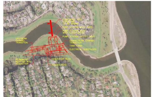
Source: USACE, Conceptual Design Report for Permanent Flood Gates and Pump Stations
