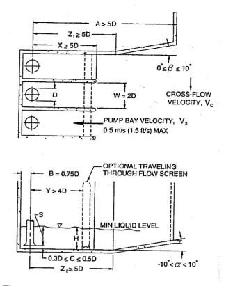
Figure 9.8.1 — Recommended intake structure layout
