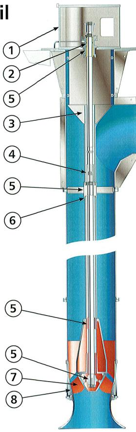
Typical section view showing pull-out type design
