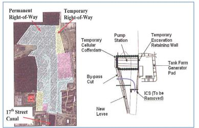
Figure 2-6. 17th Street Canal – Proposed Permanent Protection Location
