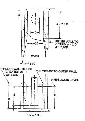
Figure 9.8.2 — Filler wall details for proper bay width
