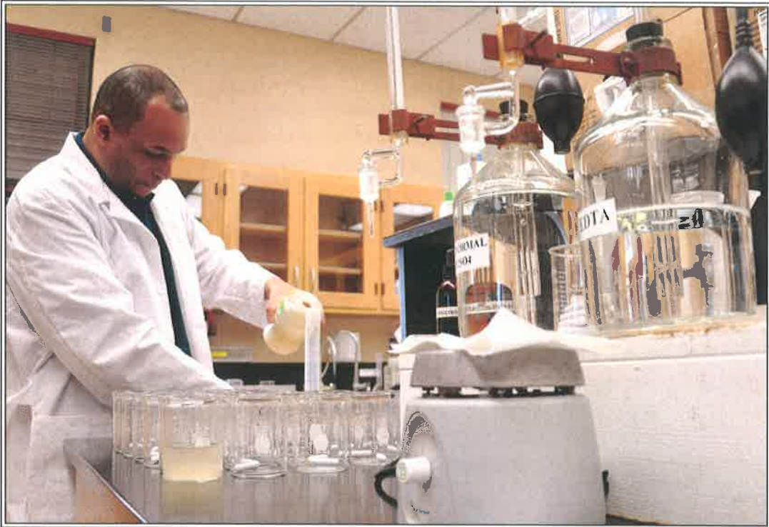
Staffed by chemists, microbiologists and technicians, the Sewerage and Water Board Water Quality Laboratory assures the safety and purity of the city's water by testing for some 150,000 organic, inorganic and microbiological compounds. The 8,500 square foot lab is located within the Carrollton Water Plant and monitors river water and finished water sampled from both the East Bank and Algiers. Pictured here, a Laboratory chemist performs water analysis.
