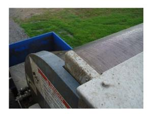
Figure 7. Drum Screen for Grease Removal
